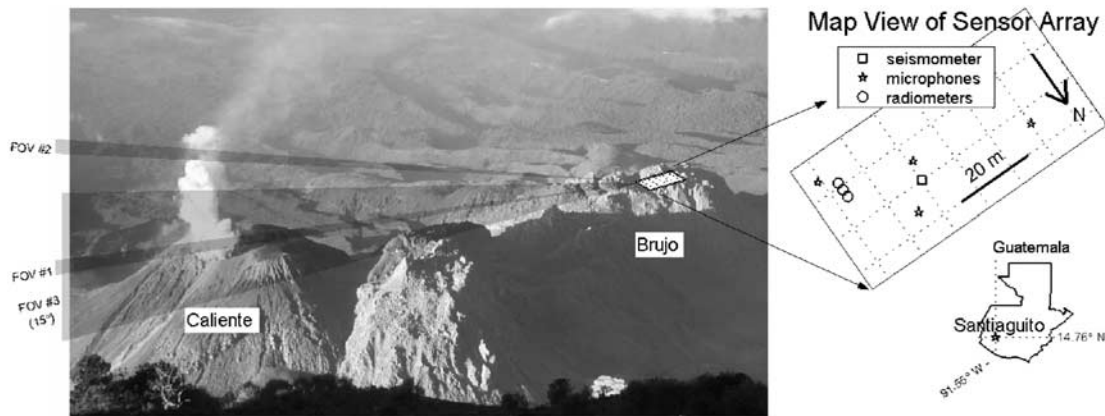
Figure 1. Santiaguito dome viewed from Santa Maria. Active Caliente vent is at left (east) \sim 1600 m from the inactive Brujo Dome, where sensors (inset map) were installed. Thermometer FOVs are shown as transparent cones.
